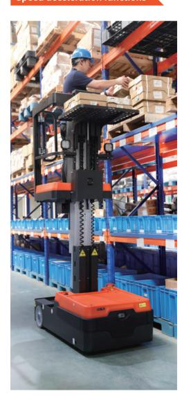
While platform is raising to its maximum height, the maximum available lift and drive speeds will go through three steps of speed settings according to the following lift height ranges for the platform: 0-500mm, 500-1500mm, 1500-3000mm to ensure the truck's stability and operator's safety.
