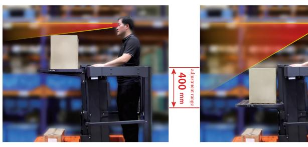
Adjustable height of the front shelf allows to ensure good visibility and avoid overlapping of operator's field of view by goods located on it.
